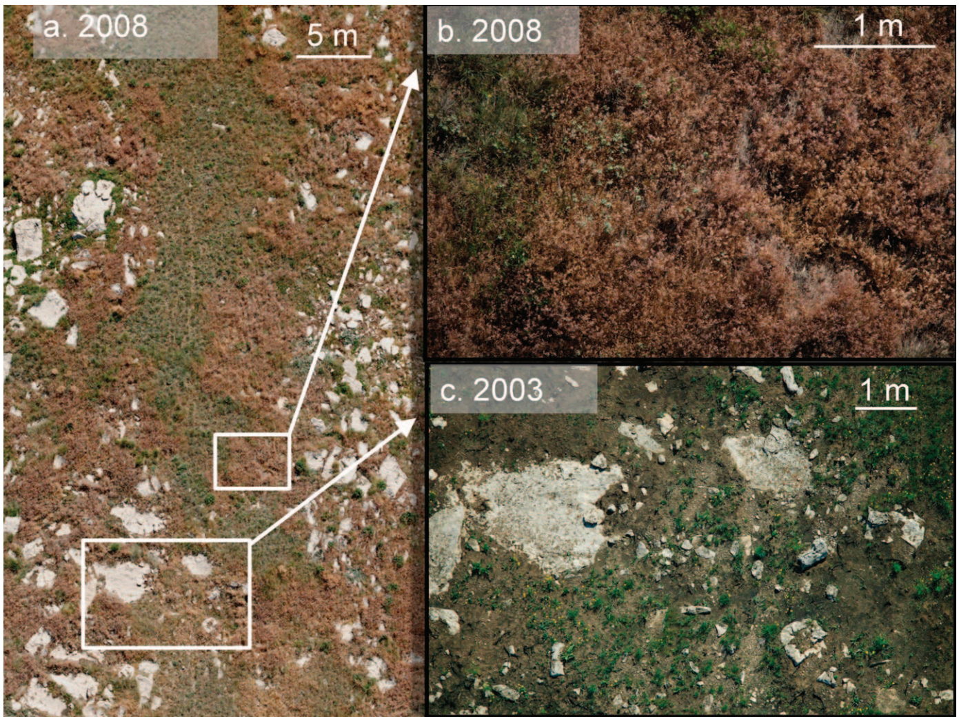
Figure 3. (a) A 17.6-mm ground sample distance (GSD) image from 2008, (b) 0.86-mm GSD image from 2008, and (c) 2.1-mm GSD image from 2003 showing overlap of aerial imagery from 2003 and 2008 at the Pass Creek no. 15 sample location. White boxes in image (a) denote locations where images (b) and (c) occur on the landscape. The rocks in the 2003 image (c) are easily recognized in the 2008 image (a). The slight lack of spatial accuracy between image (b) and image (c) may be because of GPS inaccuracy or slight tilt of the aircraft at the time of shutter release. Note that the wider field of view in image (a) shows the broad extent of downy brome at the sampling location.
